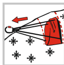
7. SNOW ANCHOR Special notches for using your shovel in this securing technique.
