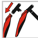
5. AXE FUNCTION For use against very compact snow (eg for snow profiling and for rutsch block tests)
